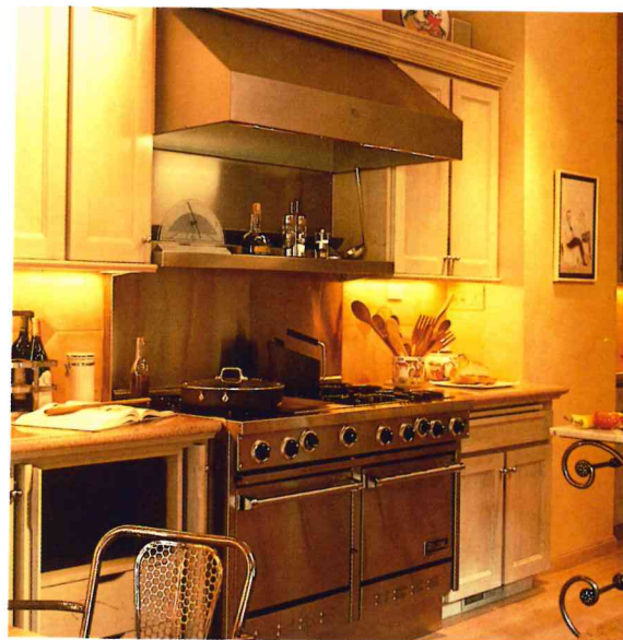
A commercial range, its sidewalls insulated for residential use, fits safely between kitchen cabinets.
